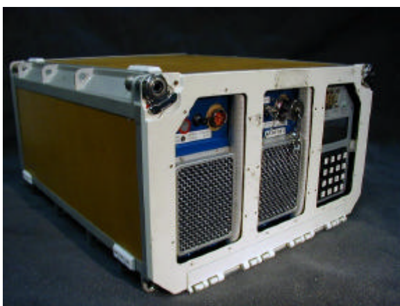
Figure 4. ICM incubator facility inside the program-provided middeck locker (composite middeck locker shown; uses metal Spacehab locker on STS-107). The insert will be removed from the locker and opened on orbit to allow manual sample processing and activations once power is turned off and cables have been disconnected.
